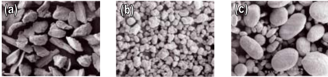
Fig. 8: A few examples of nickel coated cores for use as conductive filler materials. Nickel coated graphite ( a ); nickel coated copper ( b ) and nickel clad aluminium ( c ).
